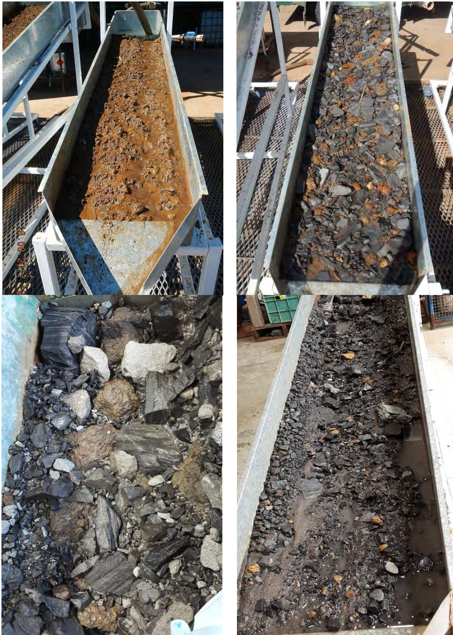
Figure 3: Red clay soil (top left), red clay soil-Fresh Permian mixture (top right), brown clay soil-sandstone mixture (bottom left), and brown clay soil-siltstone mixture (bottom right) during overland flow study.
