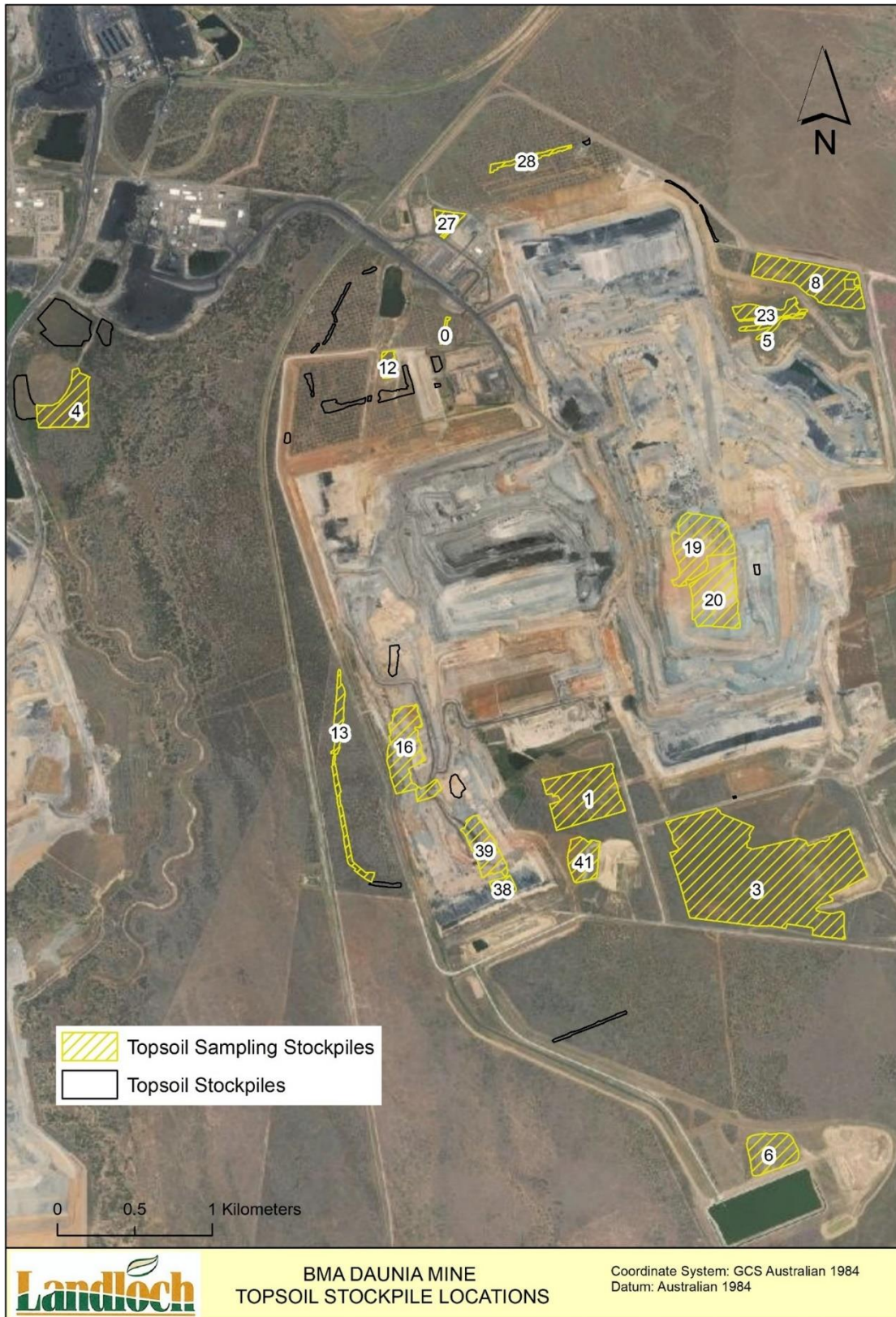
Figure A1: Distribution of stockpiled topsoil materials and sampling locations at Daunia Mine. All stockpiles sampled are representative of a singular management group.
