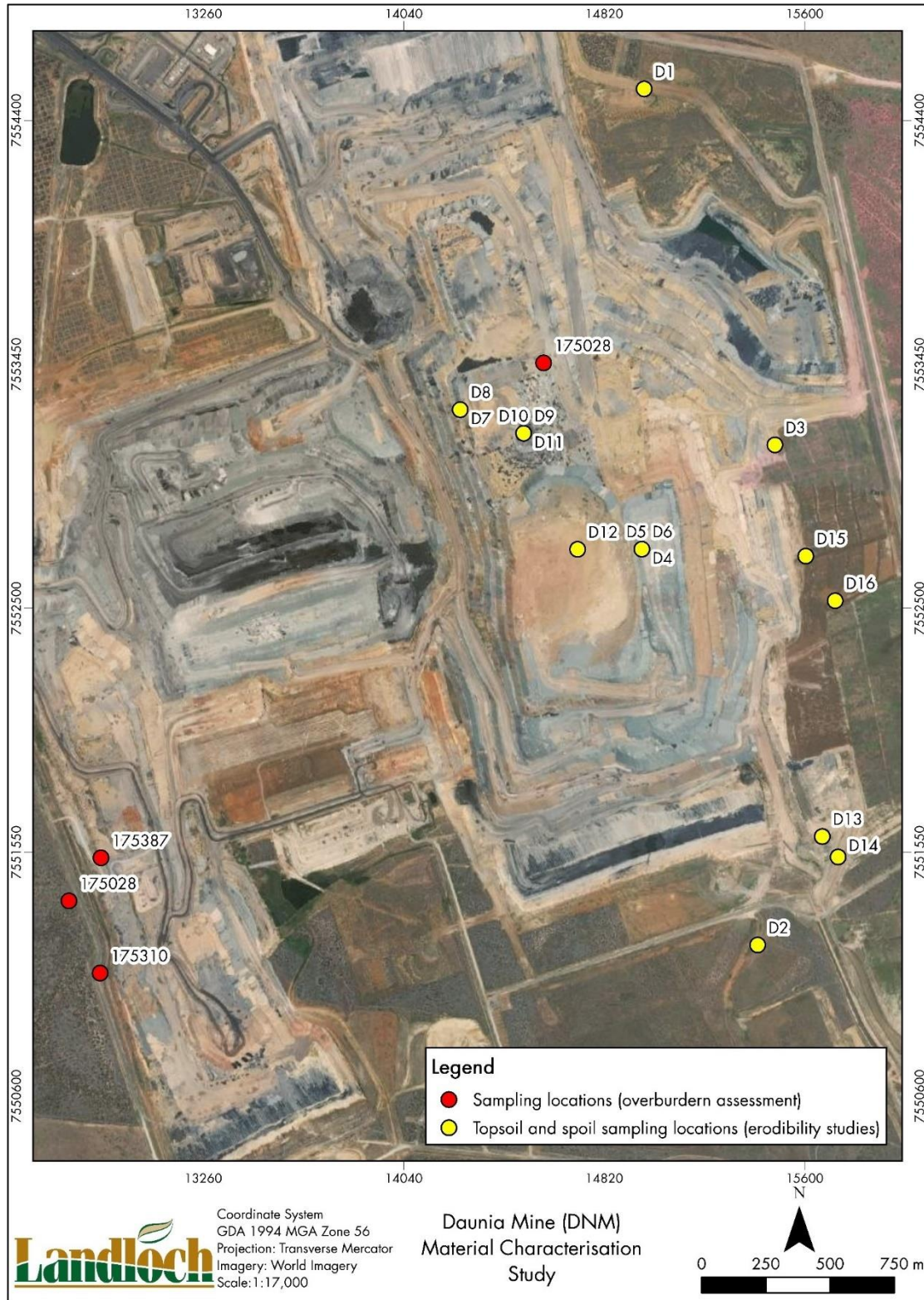
Figure A7: Topsoil and spoil sampling locations for erodibility studies (Landloch Pty Ltd, 2017) (PW Baker & Associates Pty. Ltd., 2012).
