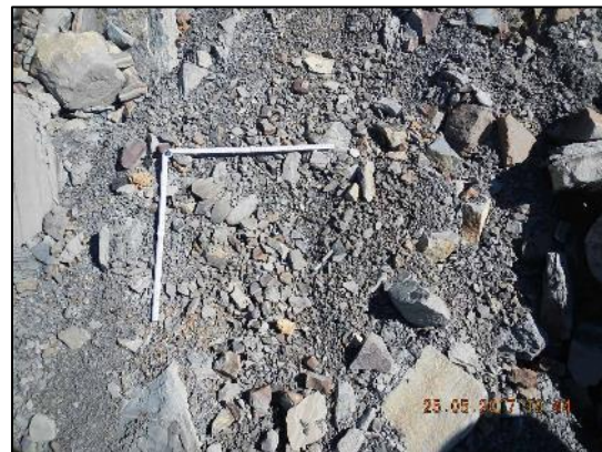
Figure 7: Permian spoil material present at Daunia Mine.
