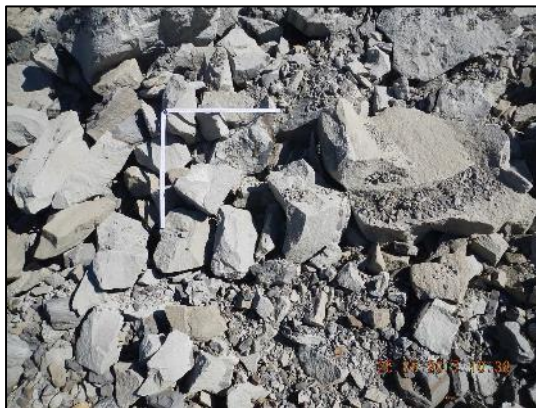
Figure 6: Fresh (<1 month) unweathered Permian sandstone spoil.
