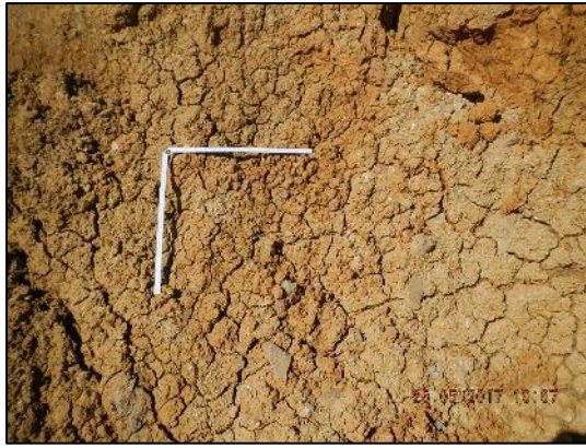
Figure 8: Weathered clay spoil material at Daunia mine.
