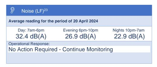
5. LF is estimated equivalent mining noise (LF = low frequency for band 20-630 HZ); Monitoring results may include noise from other sources.
