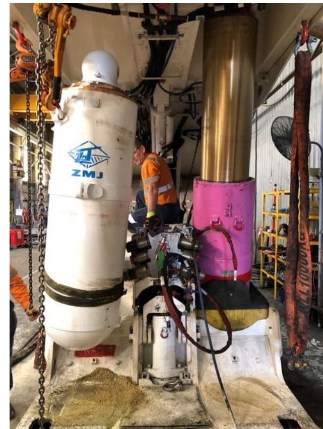
Mockup Prototype Leg Cylinder being trial fitted into existing spare Roof Support
