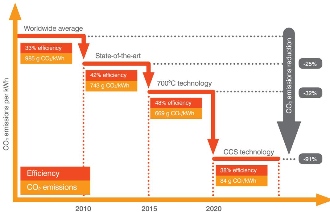
**Note:** The figure shows CO<sub>2</sub> reductions at coal-fuelled stream-electric power plants from higher efficiency / CCS technologies (hard coal, 26 GJ/kg HHV, North Sea cooling water).
