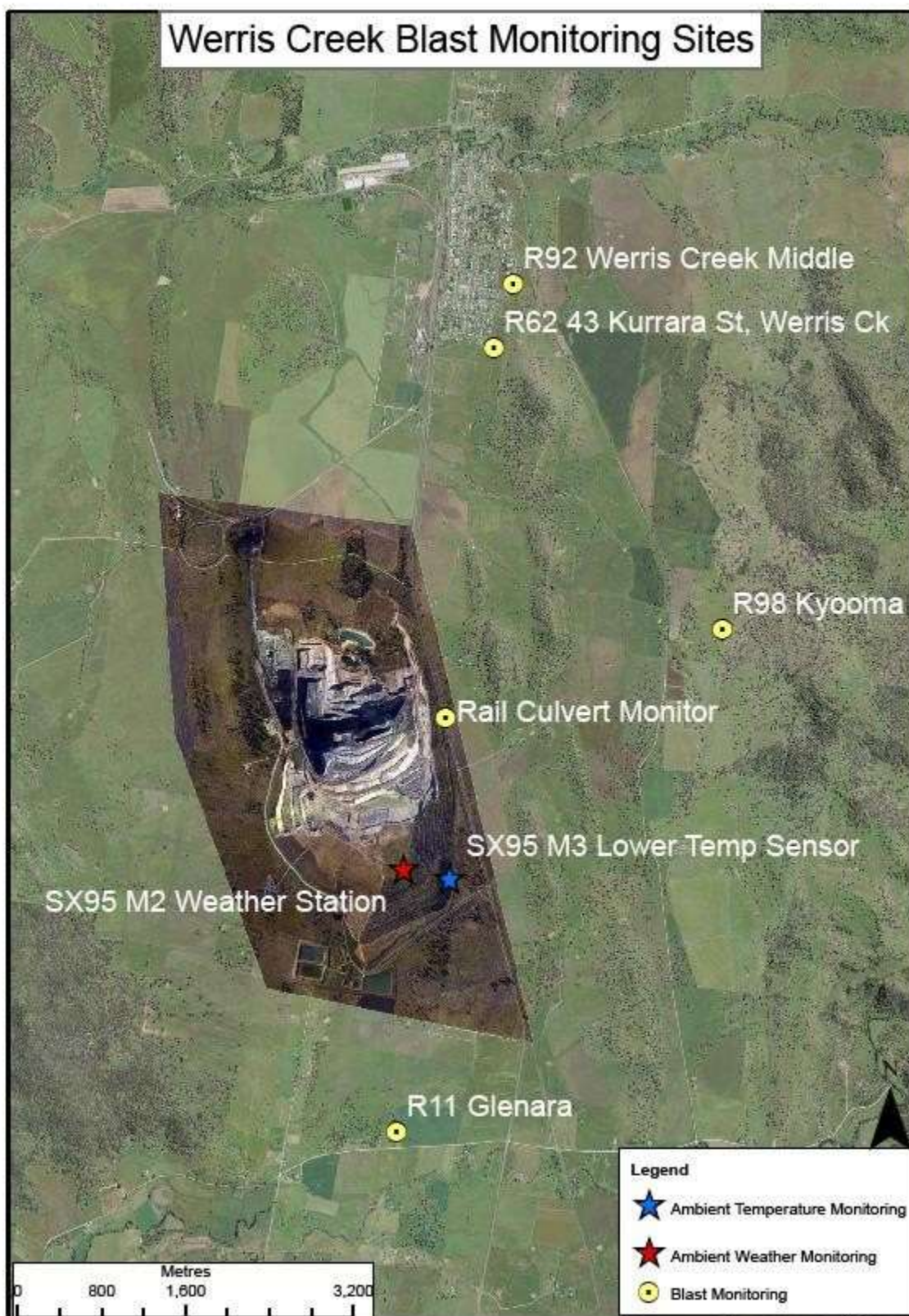
Figure 2 - Blast Monitoring Sites at WCCM
