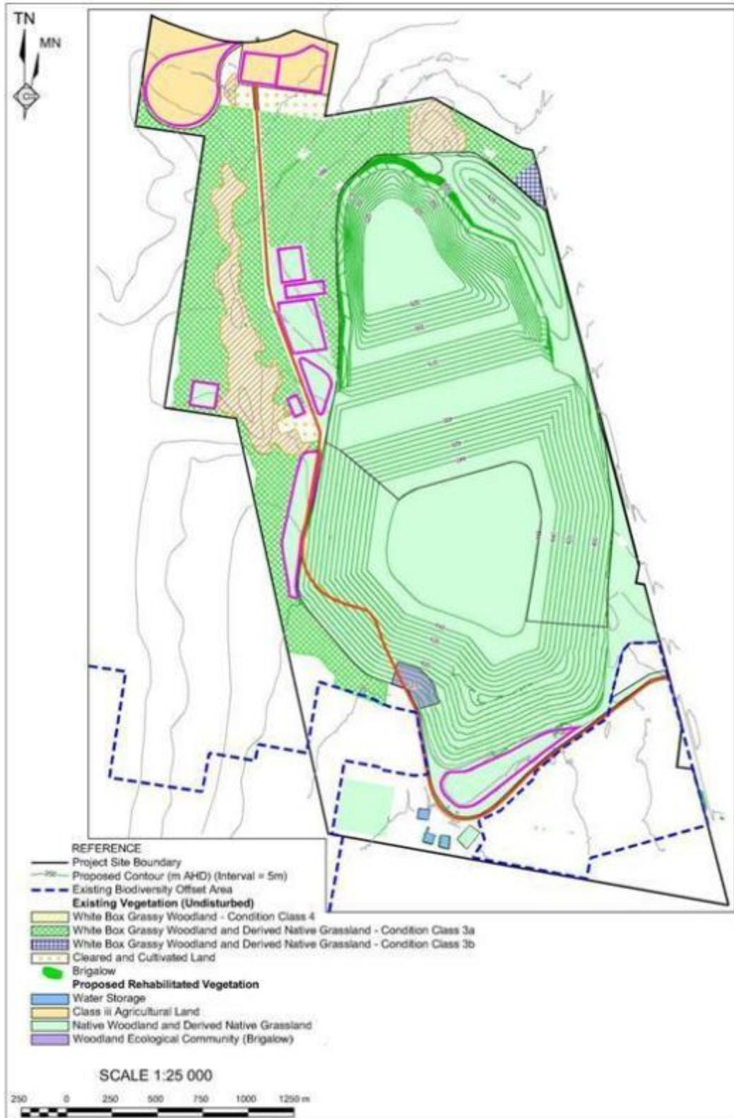
**Figure 4: Conceptual final landform and rehabilitation plan.**
