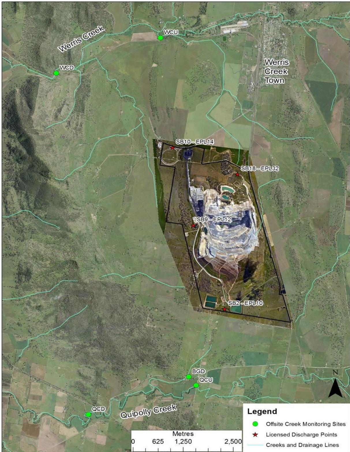
**Figure 7-2 EPL12290 Licensed Discharge Points and Offsite Creek Monitoring Locations**
