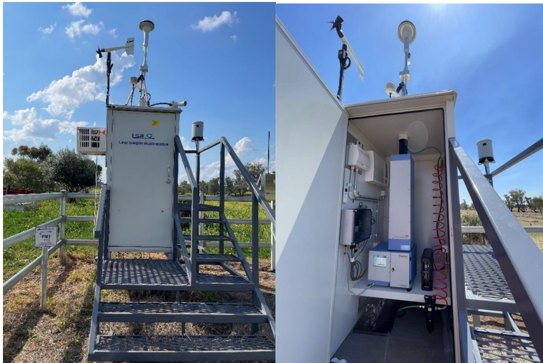
Figure 1: TEOM installed at Lanreef
