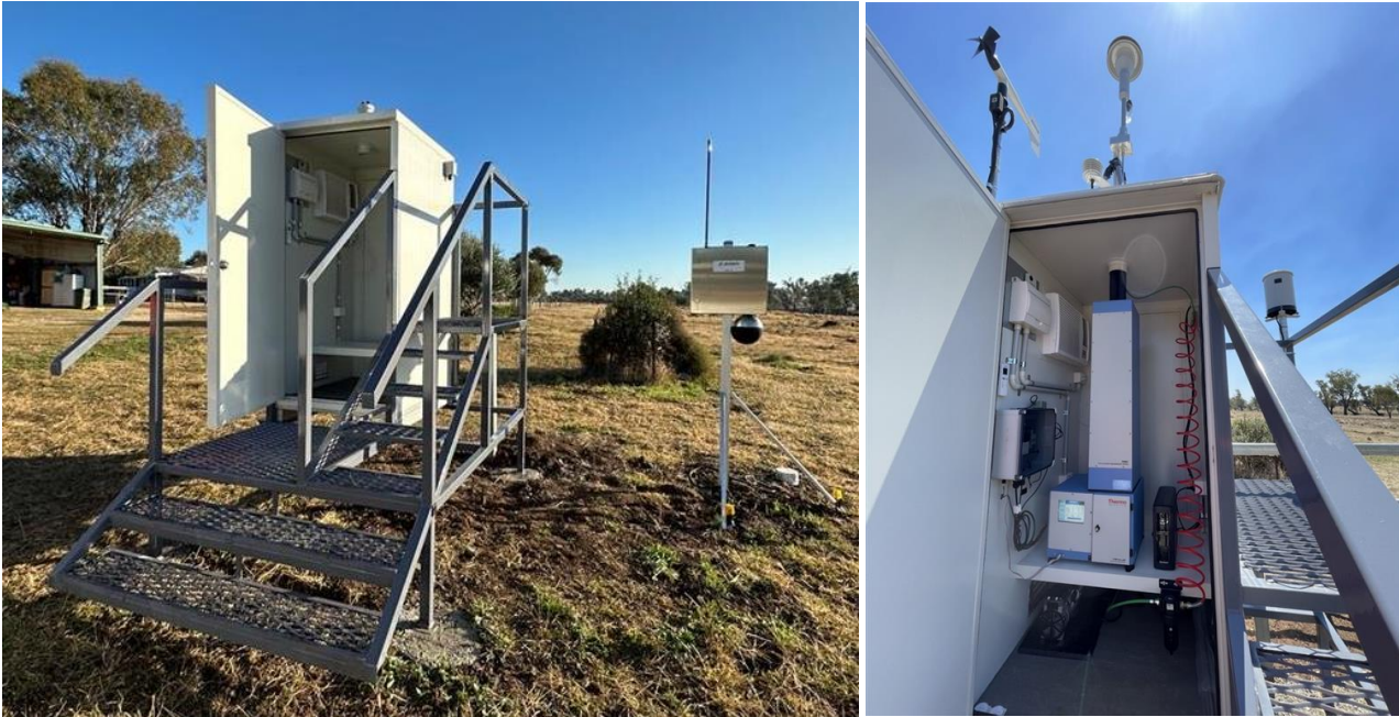
Figure 1: TEOM and blast monitor installed at Lanreef
