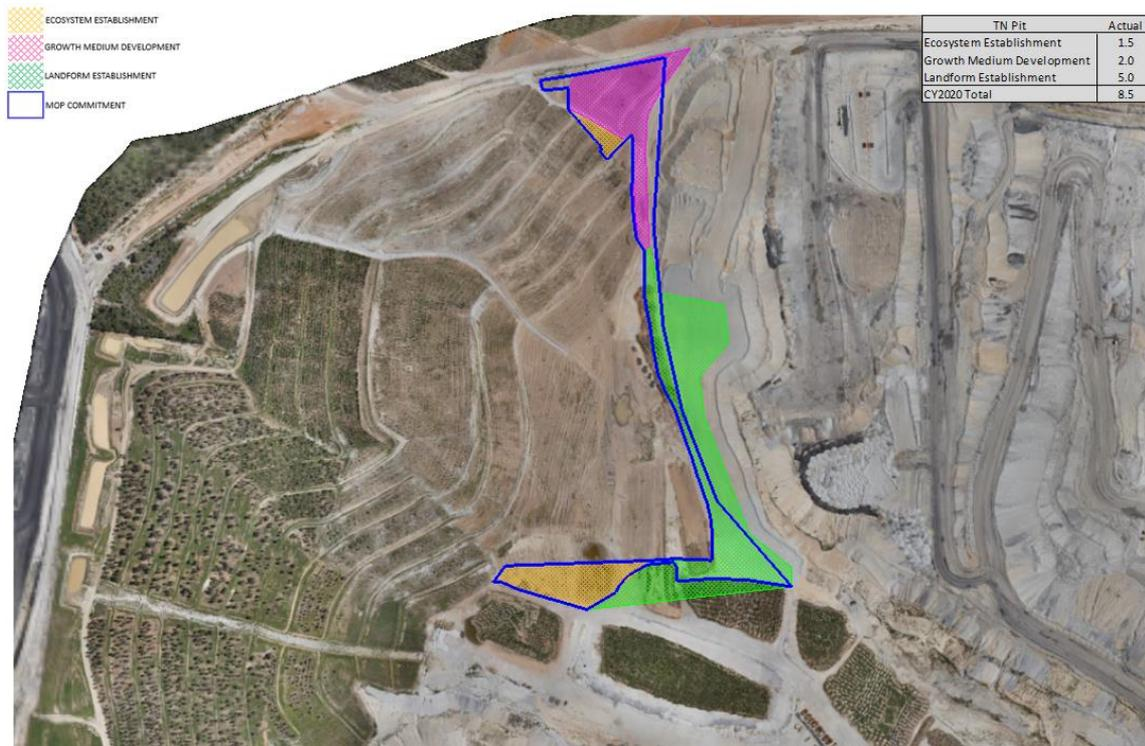
**Figure 19 - Northern Emplacement Area Rehabilitation at end of CY2020**
