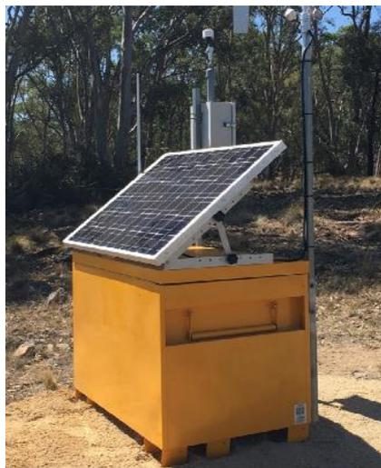
*Portable and real-time dust monitor installed at TCM in November 2018*
