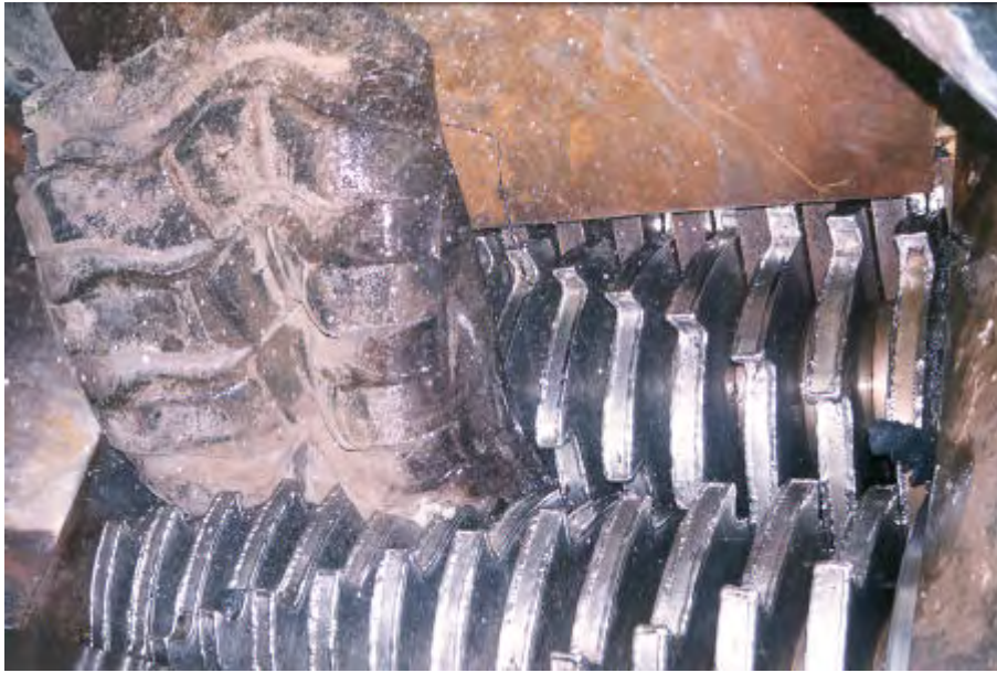
Figure 6.2.3 2300 RPM are reduced to 2 RPM through a series of gearboxes, producing high torque for shredding (NTS) (photo Matt Corbett)
