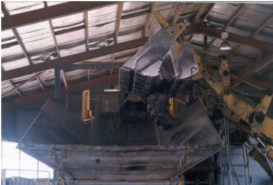
Figure 6.2.2 Feeding tyre sections into the shredder (NTS) (photo Matt Corbett)
