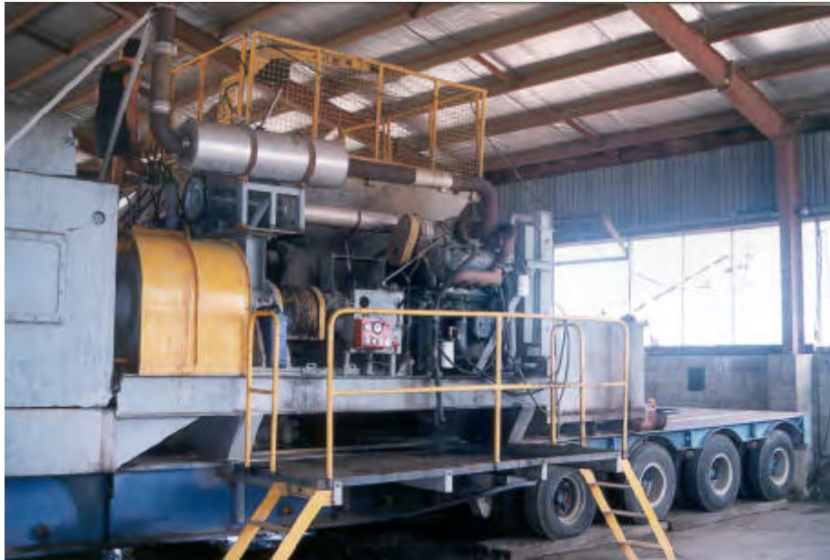
Figure 6.2.5 Northern Tyre Salvages’ mobile custom shredder (photo Matt Corbett)
