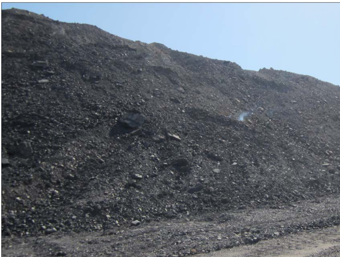
PLATE 6 Spontaneous Combustion on Overburden Emplacement
