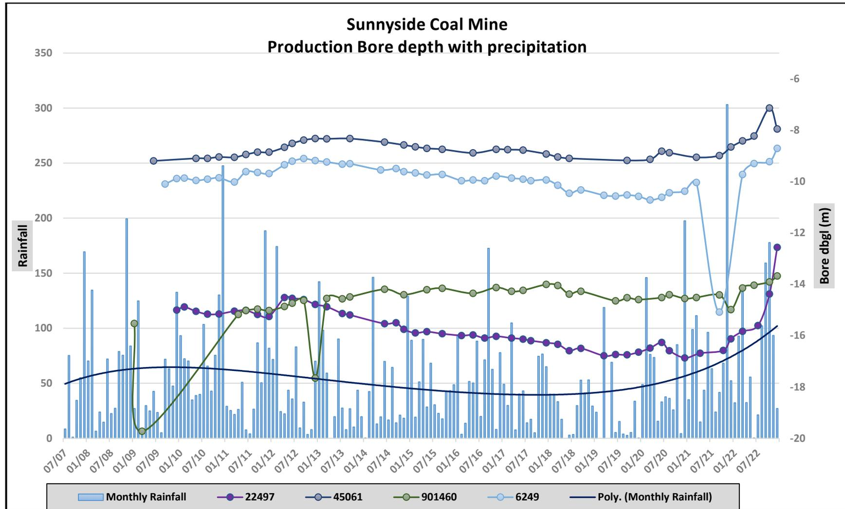
Figure 9 Production bore water depth
