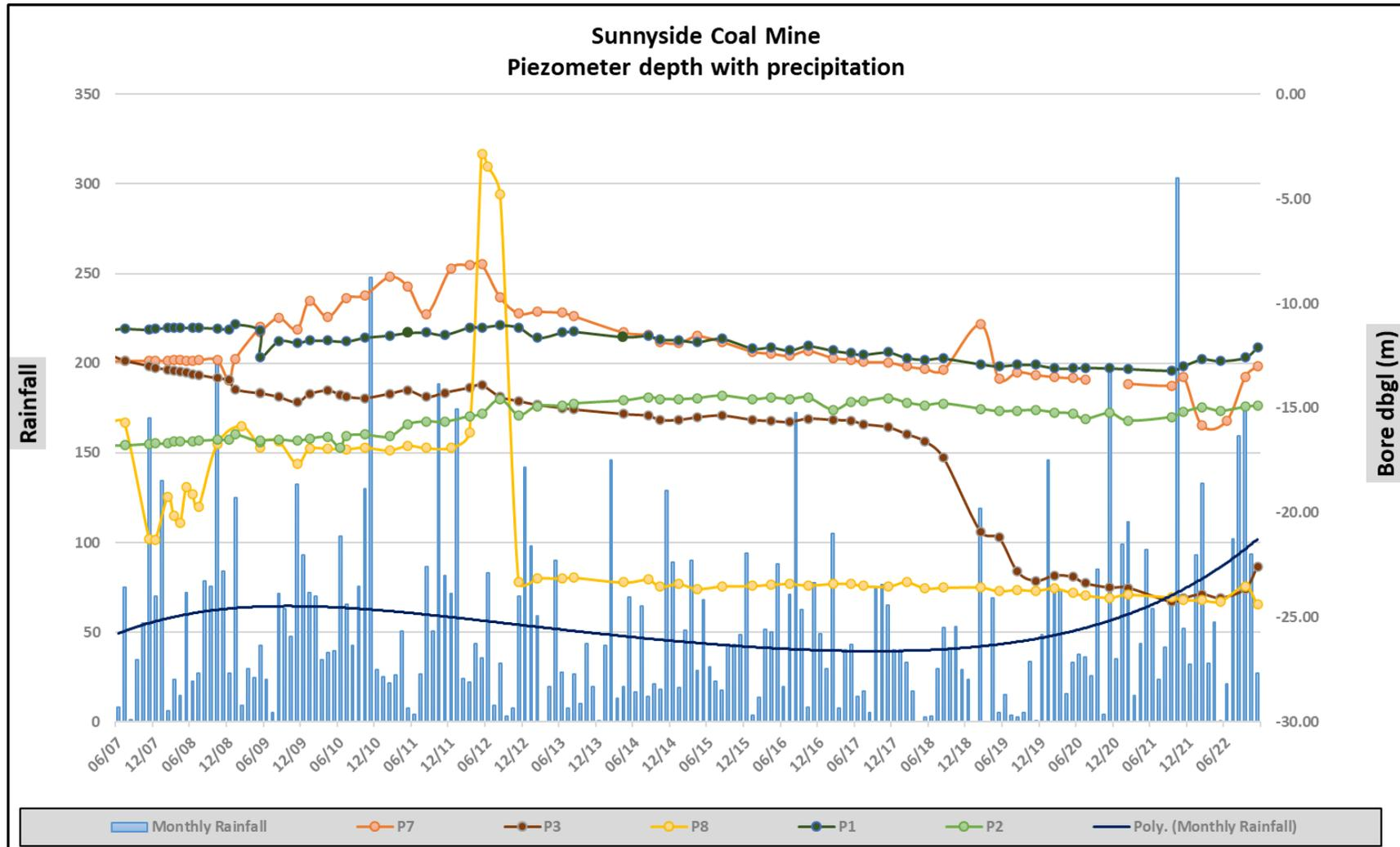
Figure 8 Monitoring piezometer water depth
