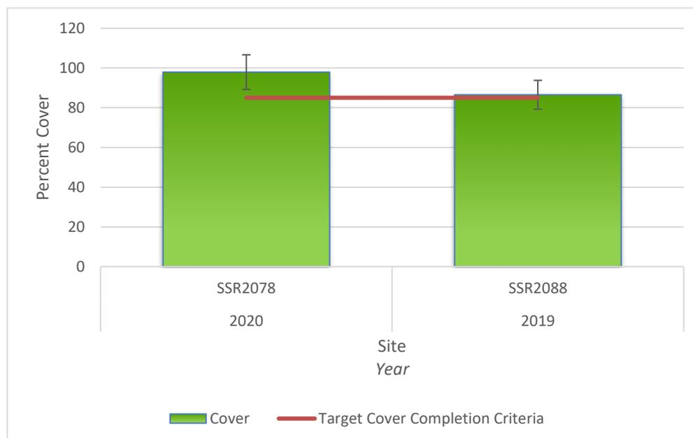
**Figure 6.2.3.4 Combined Pasture completion criteria ground cover components (vegetation, leaf litter, and mulch) at Sunnyside Mine. Line shows minimum MOP completion criteria target of 85%. Bars show standard error of the mean.**
