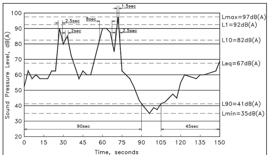
The signal in Figure 3 has a duration of 2.5 minutes (ie 150 seconds) with noises occurring as follows:
