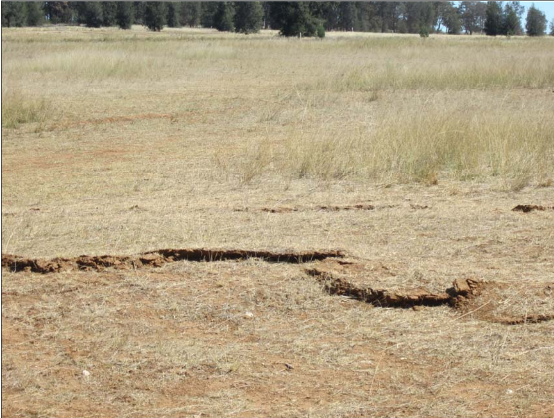
PLATE 9 Cracking associated with subsidence above LW01
