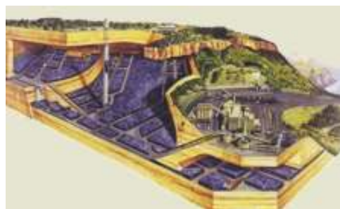
Cutaway of underground mine, south coast New South Wales, Australia (room and pillar method)
