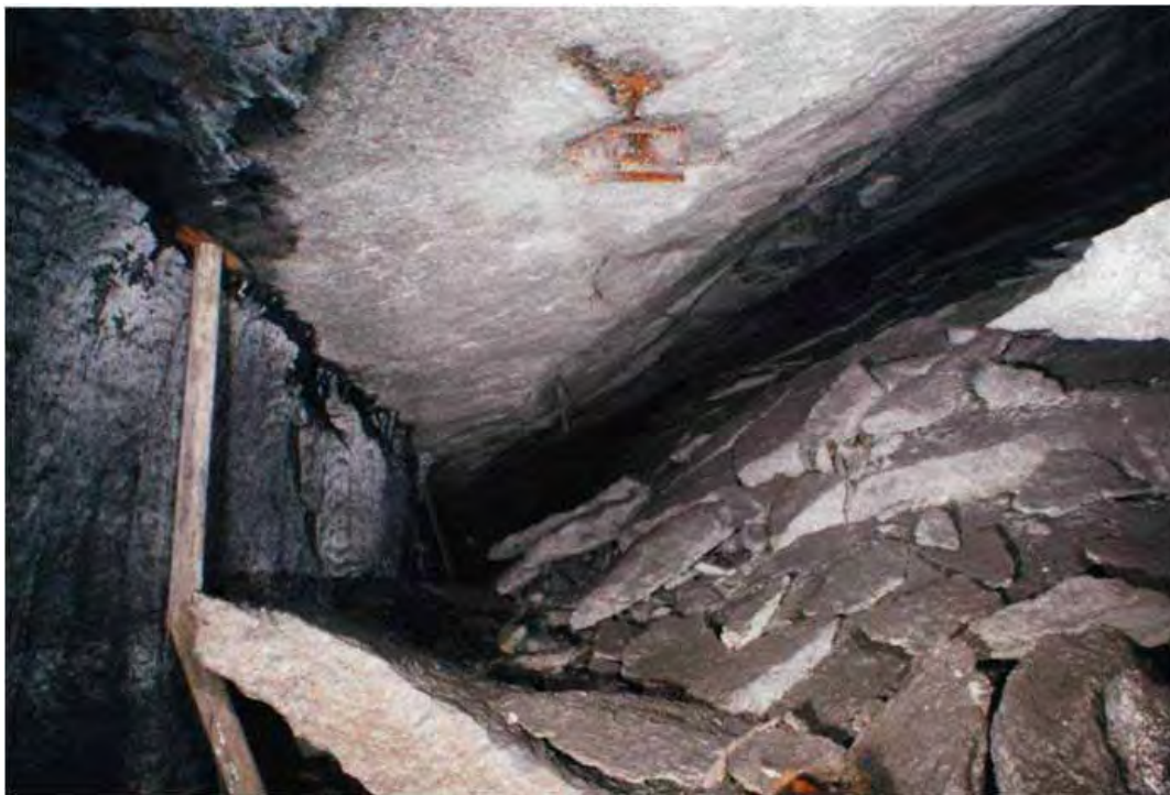
Figure 11: Example of Caving Developing Underground
