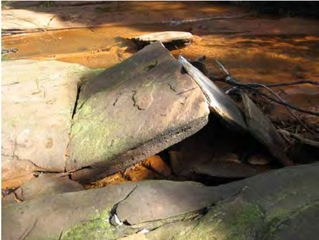
Figure 22: Buckling of Near-Surface Strata due to Upsidence, Waratah Rivulet, late 2004
