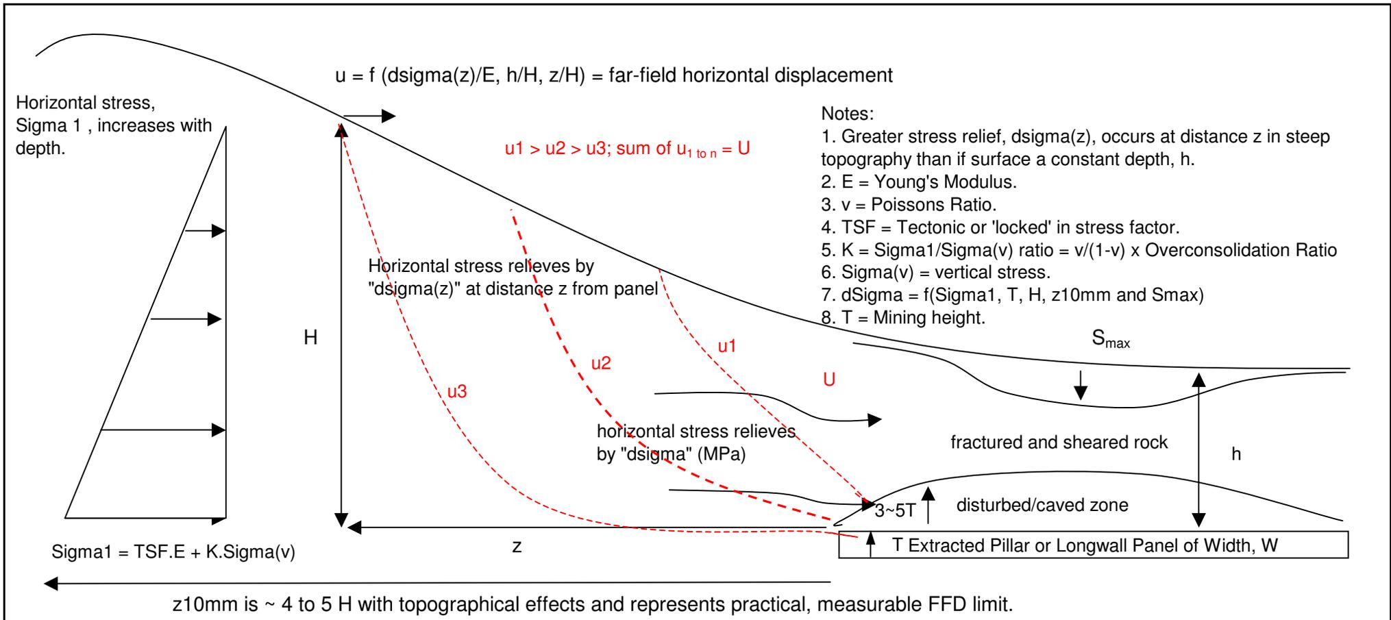
Simple Analytical Model for Predicting Total FFD :  $U = 0.5(\Sigma_1 \times 12.3/2)z_{10mm}/[E(H+h)/2] + \text{'tail' of 10mm} + S_{max}$  component (refer to text)
