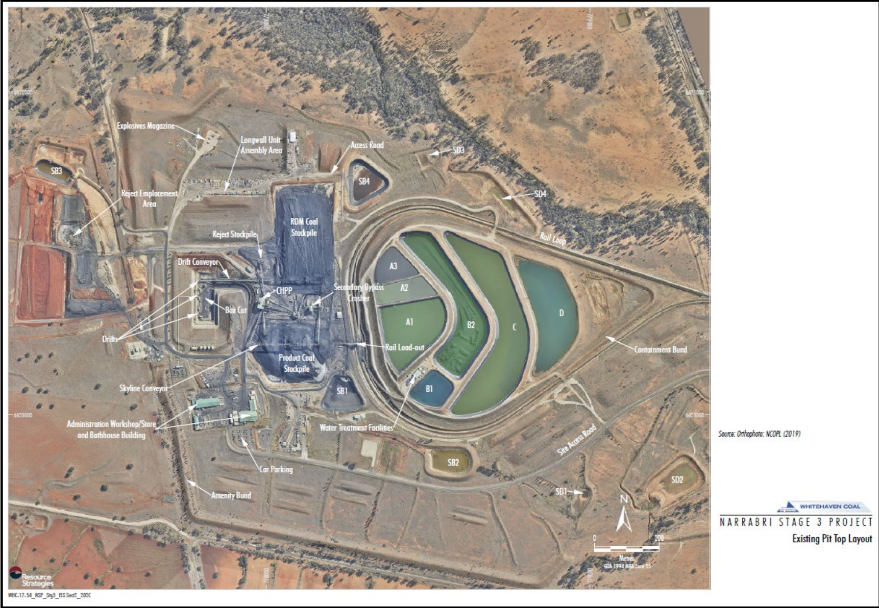
Figure 1: General Project Arrangement – Pit Top Area Narrabri Underground Mine Stage 3 Extension Project 42 (SSD-10269)
